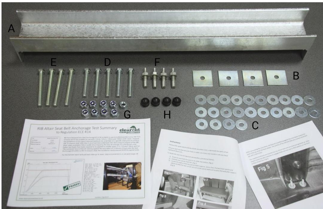
\*Anchorage/Installation tested to ECE R14 requirements. Test carried out in conjunction with 150cm 3 seater RIB Altair seat fitted into a SWB VW T5 Chassis shell. Pull Force applied exceeded 10,000kgs.
