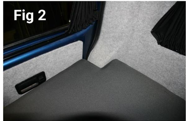
Depending on fitted floor thickness it may be necessary to tap the passenger wheel arch down with a rubber mallet. So that the frame is clear of the arch. This only needs to be tapped down by 3-5mm in the centre of the arch and does not cause any structural damage to the arch.
