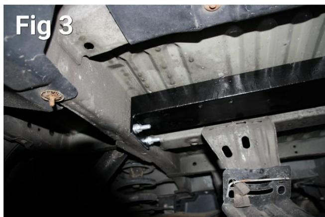
The blind bolts are inserted into the 10mm holes one at a time and tightened up. (they require a tap with a hammer to engage) Make sure you use 2 x M10 washers on the behind each nut.
