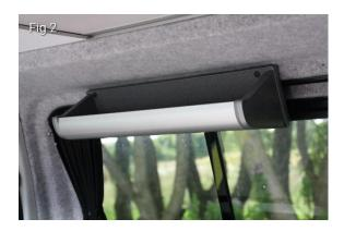
The most stable fitting positions will be those where by one side edge of the shelf is supported by either the left or right side pillar or the van. 3
